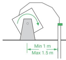
Segment entering borehole must be vertical, and not touch the casing
