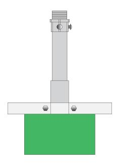
1. Assemble 27 mm ID conduit and hang it in borehole using the hanging fixture included with the SAA Install Kit. The PVC should **NOT** rest on the bottom of the borehole.
