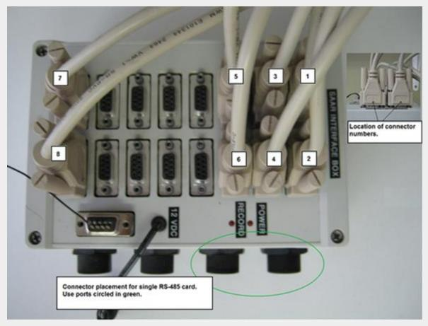
Figure 3: SAAR Interface Box cable setup for use with just a single (8-port) RS-485 card For step-by-step instruction on this process refer to the '**Connecting using the SAAR Interface Box**' Guide.
