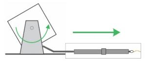
3. Remove the bell end from the conduit. Attach the rope to the eyelet on the tip end of the ShapeArray and pull it into the conduit. At the tip end, attach an end cap to the PVC. 4. Trim the PEX on the ShapeArray so that only 100 mm to 127 mm (4" to 5") is sticking out of the conduit. Loosen the compression rings on the Horizontal Installation Kit. Slide it onto the PVC casing, over the ShapeArray's cabling and PEX.
