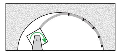
**NOTE** - Ensure only one clamp is used per segment. Clamps must be offset approximately 5 cm (2") from the bendable joints between the SAAV's segments.
