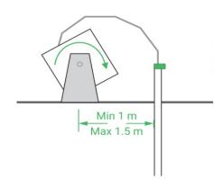
2. Place the SAAV on the reel approximately 1 m - 1.5 m (3' to 5') away from the borehole. Ensure the reel is placed such that the SAAV will come off of the reel from the top and the reel is oriented along the expected direction of movement.
