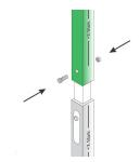
If the second Extension Tube is required, use the Extension Coupler provided in the SAAV Installation Kit to connect the tubes together.
