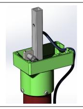
6. Set the Extension Tube Anchor on its short edge inside the Casing Cap. Apply a light amount of force on the Extension Tube (approximately 5 kg), mark a line across the top of the Extension Tube Anchor on the Extension Tube and cut along the marked line.
