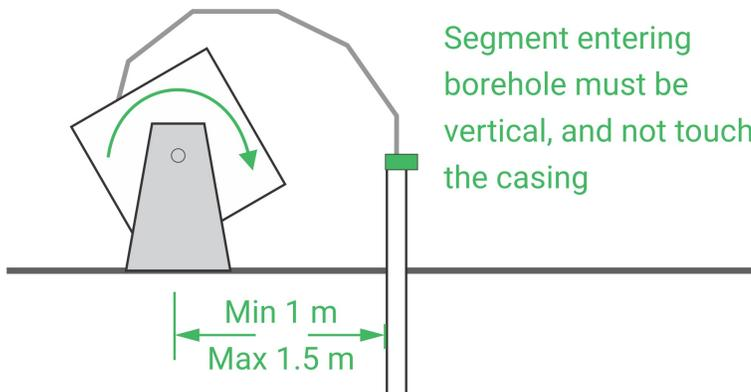
3. Place the reel stand near the borehole and lower the SAAV into the casing.
