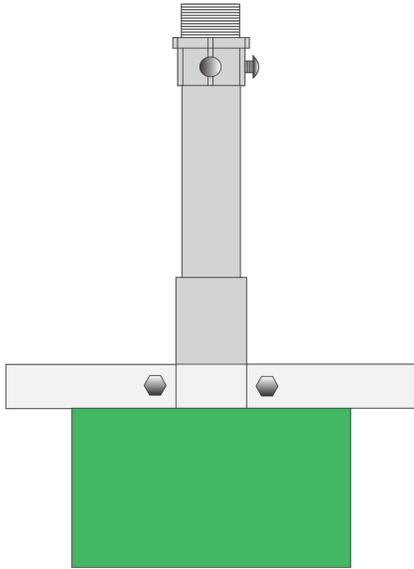
1. Assemble 27 mm ID conduit and hang it in borehole using the hanging fixture included with the SAA Install Kit. The PVC should **NOT** rest on the bottom of the borehole.
