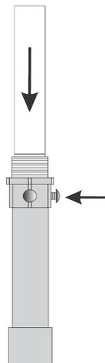
6. Compress the SAAV and tighten the set screws. Cut away excess PEX tubing and thread the top portion of the top stack onto the cabling and screw it to the bottom portion. Tighten the cable gland on the top stack to prevent moisture from entering the PVC assembly.
